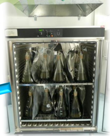
heating cabinet, 35 days, 40 C
