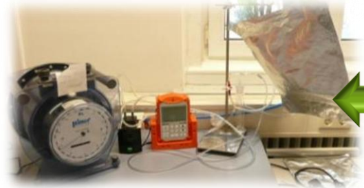
gas measuring: volume and composition
