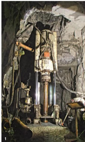
Mine operations: (1) Raise-borer; (2) Low profile loader; and (3) Jumbo.
